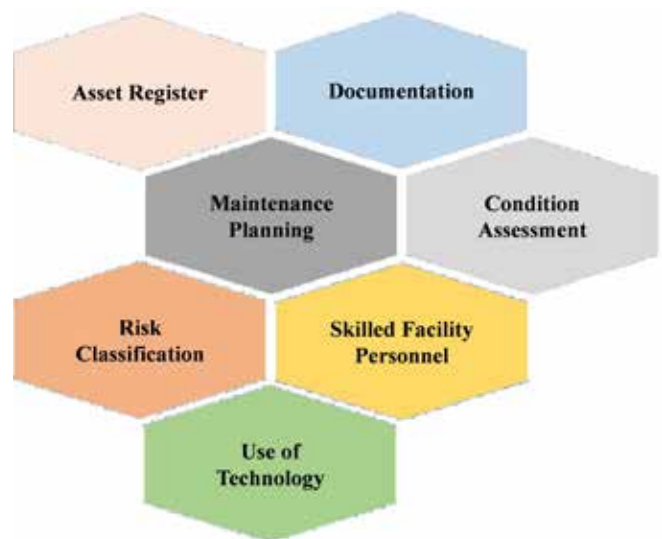
Figure 3: Key Components of an Asset Management System
