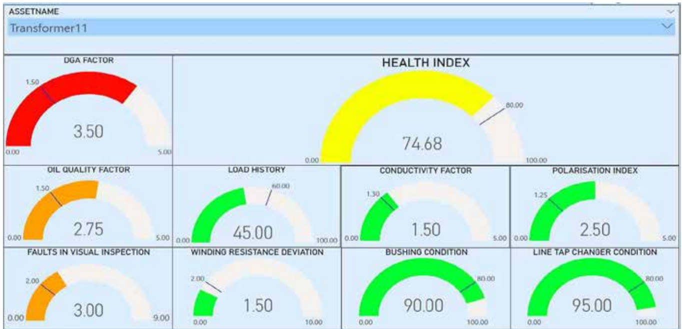
Figure 4: Health Index of a Transformer
