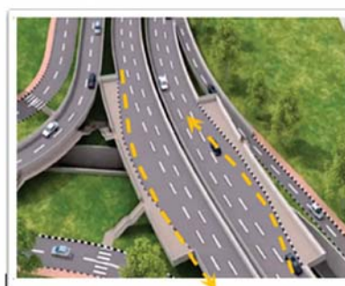
Proposed version of corridor with bus stops along the leftmost through carriageway exactly above the intersection with full pedestrian connectivity.
