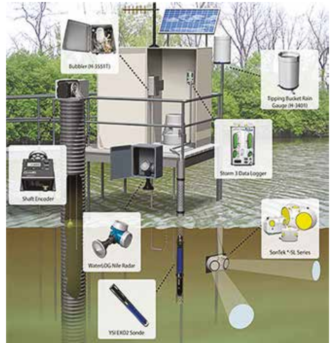
Figure 4: Water level monitoring at River (3)
