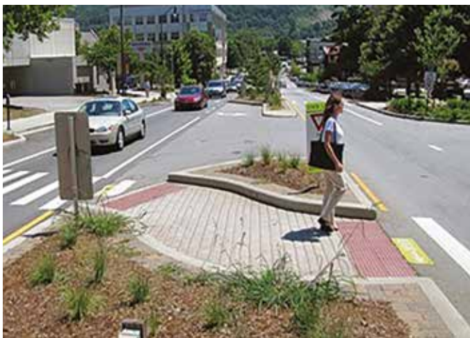
Figure 8: Median as a Refuge for Pedestrians
