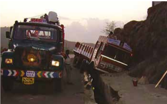
Un-protected side drains that can cause crashes.
