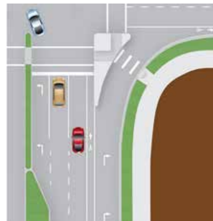
Figure 10: Traffic Channelization plus Refuge Island for Pedestrians
