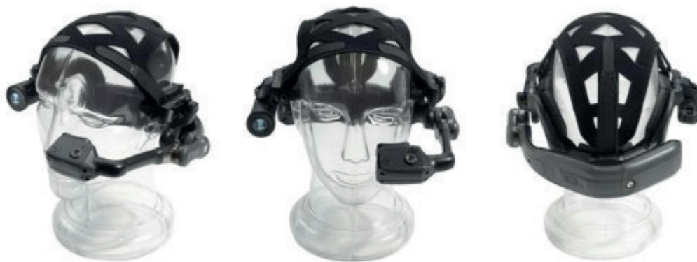
Motorola HC1 Headset Computer with voice recognition and gesture control3
