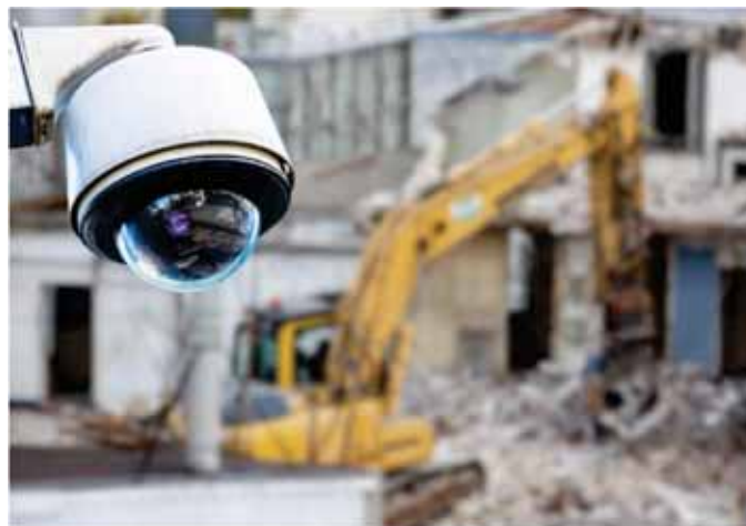
Fig.1: A PTZ camera at construction site
