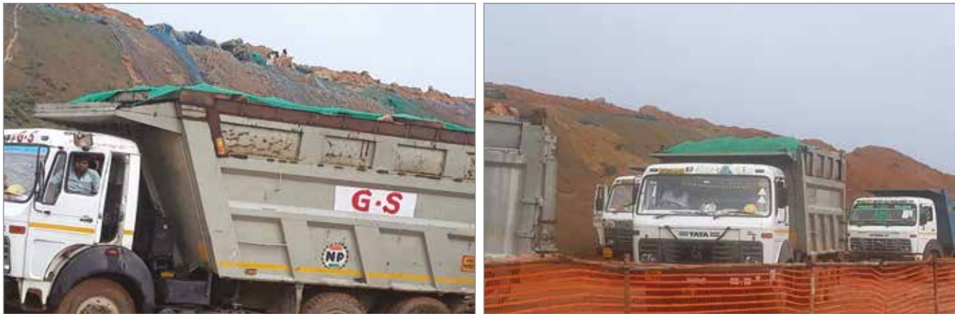
Exhibit 03: Dumpers carrying excavated material are covered
