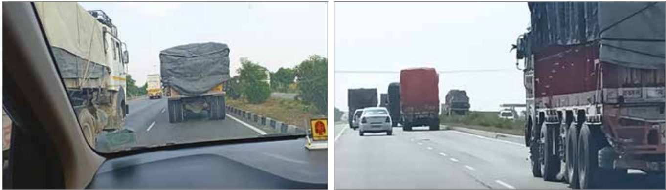
Exhibit 4A: & 4B: Illustrating the Boxing Effect by Heavy Vehicles (photos by Author)
