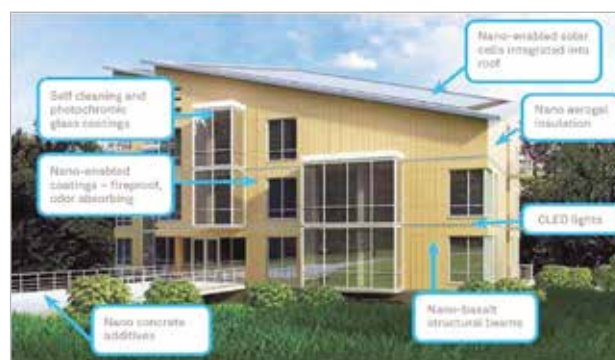
Figure 1: Energy-Efficient House of the Future [1]
