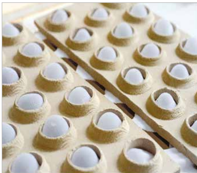
Hydro-ceramic roofing tiles [16] Courtesy of IAAC Institute for Advanced Architecture of Catalonia
