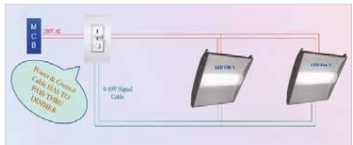
Figure 6: 1-10V Signal Dimming
