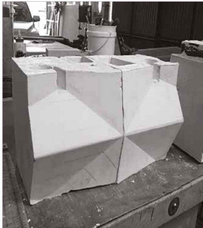
Typical View of an Air cleaning brick [12] . Courtesy: Carmen Trudell Assistant Professor -at School of Architecture Cal Poly San Luis Obispo
