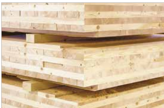
Mass timber- Laminated panels [4] Courtesy: FPInnovations
