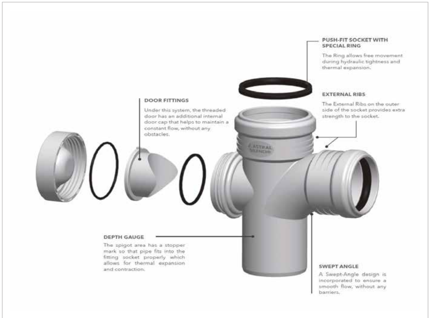
Figure 2: Fitting for Polypropylene SWR pipes
