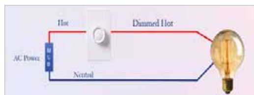
Figure 3: Phase Dimming by Dimmer
