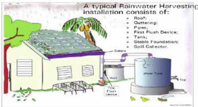
Figure-2: Typical RWH Installations in Maldives Source: Design of RWH in Maldives
