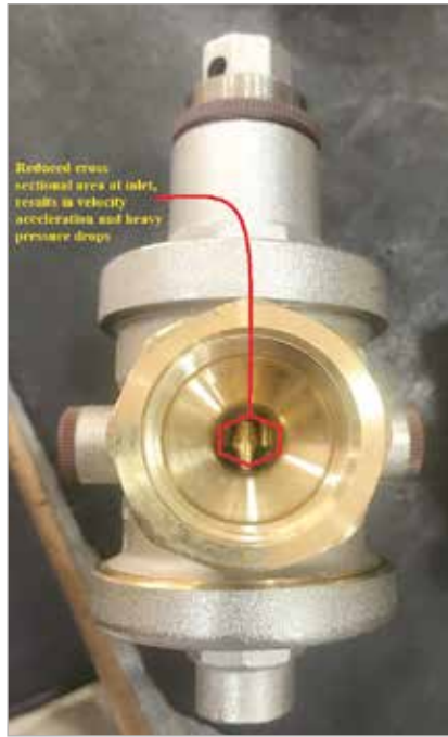
Figure-2: Piston PRV with reduced ports
